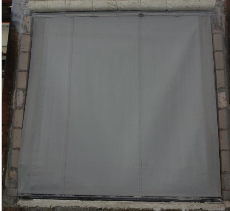
Fig. 9 Exposed Side after Temperature/Time Resistance Test
