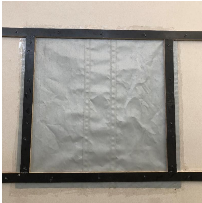
Fig. 2 The curtain material during Permeability to Smoke Test
