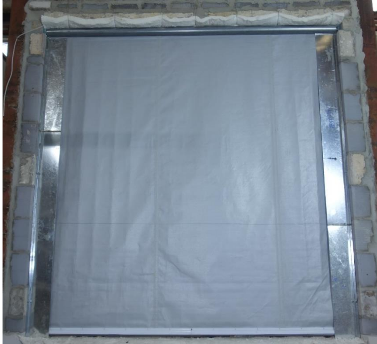
Fig. 3 Unexposed Side Prior to Temperature/Time Resistance Test
