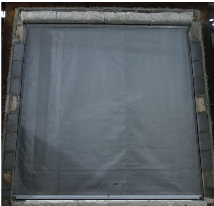
Fig. 4 Exposed Side Prior to Temperature/Time Resistance Test
